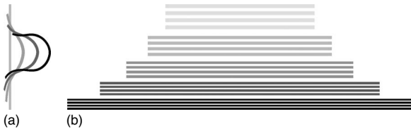
FIG. 2. (a) Bending of a material line. (b) Evolution of a striated structure in a pure strain region. Temporal evolution from light gray to black.
